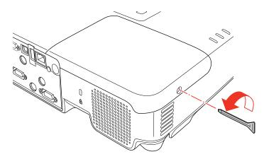
**Warning:** If the lamp is broken, glass fragments may be loose inside the lamp chamber. Be careful removing any broken glass to avoid injury.
